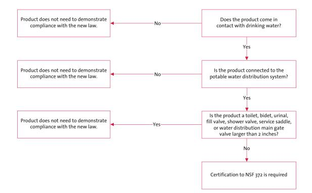
These requirements cover the evaluation of wetted surfaces of products, components, and materials that convey or dispense water that is intended for human consumption by drinking or cooking for lead (Pb) content.
